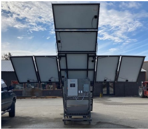
Figure 3 Fully Deployed Rear View Showing Discharging Components
